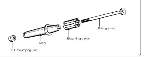
When placing an order for arbors and expanding sleeves, please provide the order codes individually. They will be shipped without being assembled.
